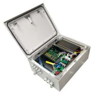
**High performance gigabit switch.** The key element of the switch is high performance chip from Marvell, which is able to process a large volume of traffic coming from the IP cameras.
