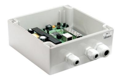
**TFortis PSW-11** — unmanaged switch. It is designed for locating a single IP camera over a long distance. It has 1 port 10/100Base-Tx PoE with RJ-45 connector and 1 port SFP 100/1000 Base-X. It is made in a hermetic casing IP66. Operation temperature is -  $55^{\circ}$  C to +  $50^{\circ}$  C (- $67^{\circ}$ F to  $122^{\circ}$ F).
